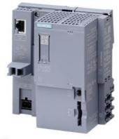
SIMATIC DP, CPU 1510SP F-1 PN for ET 200SP, central processing unit with 300 KB work memory for program and 1 MB for data, 1st interface: PROFINET IRT with 3-port switch, 6 ns bit performance, SIMATIC Memory Card required, BusAdapter required for port 1 and 2
