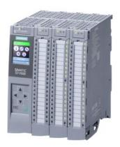
SIMATIC S7-1500 compact CPU CPU 1512C-1 PN, central processing unit with work memory: 400 KB for program and 2 MB for data, 32 digital inputs, 32 digital outputs, 5 analog inputs, 2 analog outputs, 6 high-speed counters, 4 high-speed outputs for PTO/PWM/frequency output, 1st interface: PROFINET IRT with 2-port switch, 25 ns bit performance, including push-in front connector, SIMATIC Memory Card required
