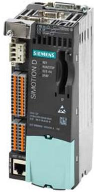
SIMOTION Drive-based Control Unit D410-2 DP; programmable single-axis motion controller with multi-axis option; interfaces: 5 DI, 8 DI/DO, 3 F-DI, 1 F-DO, 1 AI, 1 encoder, 1 DRIVE-CLiQ, 2 PROFIBUS, 1 ethernet
