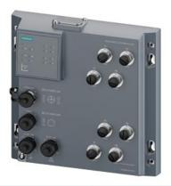
SCALANCE XP208PoE EEC, IP65, managed layer 2 IE switch, IEC 6 2443-4-2 certified; 6x 10/10 0 Mbps, 2x 1000 Mbps, M12 ports, 802.3 at 8x30 W (max. 240 W) LED diagnostics, error signaling contact, redundant power supply, PROFINET IO device, network management, can be operated in redundant ring, dust caps, including -40 °C to +70 °C, C-PLUG optional.
