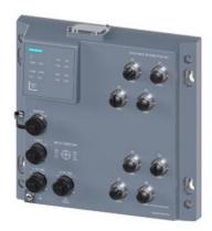
SCALANCE XP208G PoE EEC, IP65, layer 2 IE switch, 8x 100/1000 Mbps, M12 ports, 802.3at, 8x30 W (max. 240 W), LED diagnostics, error signaling contact, redundant power supply, PROFINET IO device, network management, can be operated in redundant ring, dust caps, including -40 °C to +70 °C C-PLUG optional.
