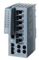
SIPLUS NET SCALANCE XC206-2 based on 6GK5206-2BB00-2AC2 with conformal coating, -40...+70 °C, manageable layer 2 IE switch; 6x 100 Mbps RJ45 ports; 2x 100 Mbps ST/BFOC ports; 1x console port; diagnostics LEDs redundant power supply temperature range -40 °C to +70 °C; assembly: DIN rail/S7 mounting rail/wall redundancy functions; office features (RSTP, VLAN,etc.); PROFINET IO device; Ethernet/IP-compliant C-Plug slot;
