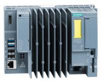
SIMATIC ET 200SP Open Controller, CPU 1515SP PC2 TF, 8 GB RAM (basic device 6ES7677-2DB40-0AA0), 128 GB CFast with Windows 10 IoT Enterprise LTSC 2019 64-bit and S7-1500 Failsafe Software Controller CPU 1505SP TF V2x preinstalled; interfaces: 1x slot CFast, 1x slot SD/MMC, 1x connection for ET 200SP BusAdapter PROFINET, 1x 10/100/1000 Mbps Ethernet, 2x USB 3.0, 2x USB 2.0, 1x DisplayPort; documentation on CFast, restore image on CFast
