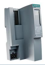
SIPLUS ET 200SP IM155-6PN ST BA TX rail based on 6ES7155-6AA01-0BN0 with conformal coating, -40...+70 °C, OT4 with ST1/2 (+85 °C for 10 minutes), bundle PROFINET IM, 1 slot for BusAdapter, max. 32 I/O modules and 16 ET 200AL modules, single hot swap, bundle consists of: interface module (6AG2155-6AU01-4BN0), server module (6AG1193-6PA00-7AA0), BusAdapter BA 2xRJ45 (6AG2193-6AR00-4AA0)
