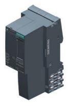
SIPLUS ET 200SP IM155-6PN ST BA based on 6ES7155-6AA01-0BN0 with conformal coating, -40...+70 °C, bundle PROFINET IM, 1 slot for BusAdapter, max. 32 I/O modules and 16 ET 200AL modules, single hot swap, bundle consists of: interface module (6AG1155-6AU01-7BN0), server module (6AG1193-6PA00-7AA0), BusAdapter BA 2xRJ45 (6AG1193-6AR00-7AA0)
