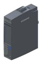
SIPLUS ET 200SP AI 8xRTD/TC 2-wire based on 6ES7134-6JF00-0CA1 with conformal coating, -40...+60  $^{\circ}$ C, analog input module, suitable for BU type A0, A1, color code CC00, channel diagnostics, 16-bit, +/-0.1%
