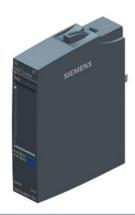
SIPLUS ET 200SP AI 4xU/I 2-w ST based on 6ES7134-6HD01-0BA1 with conformal coating, -40...+70  $^{\circ}$ C, analog input module, suitable for BU type A0, A1, color code CC03, module diagnostics, 16 bit, +/-0.3%
