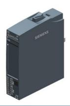
SIPLUS ET 200SP DQ 16x24VDC/ 0.5A TX rail based on 6ES7132-6BH01-0BA0 with conformal coating, -40...+70 °C, OT4 with ST1/2 (+85 °C for 10 minutes), digital output module, suitable for BU type A0, color code CC00, source output (PNP,sourcing output) substitute value output, module diagnostics for: short circuit to L+ and M, wire break, supply voltage
