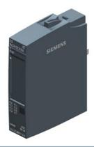
SIPLUS ET 200SP DQ 8x24VDC/0.5A Standard based on 6ES7132-6BF01-0BA0 with conformal coating, -40...+70  $^{\circ}$ C, digital output module, suitable for BU type A0, color code CC02, channel diagnostics,
