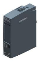
SIPLUS ET 200SP DQ 8x24VDC/0.5A HF based on 6ES7132-6BF00-0CA0 with conformal coating, -40...+70  $^{\circ}$ C, digital output module, suitable for BU type A0, color code CC02, channel diagnostics,
