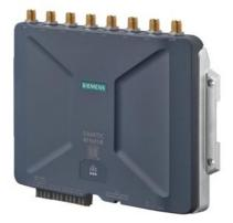
SIMATIC RF600 Reader RF695R CMITT; interface Ethernet RJ45 PoE 8 antennas, 1 digital input/ 1 digital output, 24 V DC; -25 to +55  $^{\circ}$ C; without accessories and antennas.
