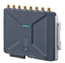
SIMATIC RF600 Reader RF695R FCC; Ethernet RJ45 PoE 8 antennas, 1 DI/DQ, 24 V DC; -25 to +55 °C; without accessories and antennas.
