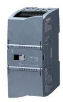
SIPLUS S7-1200 SM 1232 4AQ based on 6ES7232-4HD32-0XB0 with conformal coating, -20...+60 °C, SIMATIC S7-1200, analog output, SM 1232, 4 AQ, +/-10 V, 14-bit resolution, or 0-20 mA, 13-bit resolution
