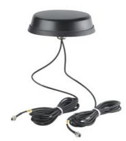
ANT897-1NY mobile wireless antenna for public and private 5G/4G/3G/2G mobile networks with 2 antenna elements; omnidirectional characteristic 700..4200 MHz; antenna gain: 0-2 dBi, including 2x 3 m cable with SMA male connection, color: black IP69K; -30..+70 °C; observe national approvals; mounting on non-conductive surface on roof and vehicle information sheet as hard copy German/English.
