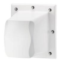
ANT897-5FF antenna for private 5G mobile networks with 4 antenna elements and weak directional effect 3400.. 4200 MHz; antenna gain: 9 dBi, including 4xN-Connect female connection IP66; -40..+80 °C; observe national approvals; scope of delivery: 1x ANT897-5FF, fixing accessories for mounting on mast and rail, information sheet en/de
