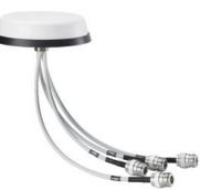
ANT897-5PN antenna for private 5G mobile networks and WLAN with 4 antenna elements; omnidirectional characteristic; 2.3..7.2 GHz; antenna gain: 4..6dBi, including 4x cables with N-Connect female connection staggered length 20..27 cm; IP69K; -30..+70 °C; observe national approvals; mounting on roof, vehicle and ceiling; information sheet as hard copy German/English.
