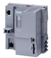
SIMATIC DP, CPU 1512SP F-1 PN for ET 200SP, central processing unit with 600 KB work memory for program and 2 MB for data, 1st interface: PROFINET IRT with 3-port switch, 6 ns bit performance, SIMATIC Memory Card required, BusAdapter required for port 1 and 2
