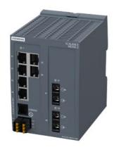
SCALANCE XB206-2 managed Layer 2 IE switch 6x 10/100 Mbps RJ45 ports 2x MM FO SC port 1x console port, diagnostics LED redundant power supply; IEC 62443-4-2 certified; temperature range 0 °C to +60 °C; DIN-rail mounting; default PROFINET.
