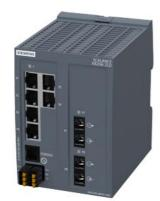
SCALANCE XB206-2LD managed Layer 2 IE switch 6x 10/100 Mbps RJ45 ports 2x SM FO SC port 1x console port, diagnostics LED redundant power supply; IEC 62443-4-2 certified; temperature range 0 °C to +60 °C; DIN-rail mounting; default PROFINET.
