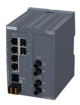
SCALANCE XB206-2 managed Layer 2 IE switch 6x 10/100 Mbps RJ45 ports 2x MM FO ST port 1x console port, diagnostics LED redundant power supply; IEC 62443-4-2 certified; temperature range 0 °C to +60 °C; DIN-rail mounting; default PROFINET.
