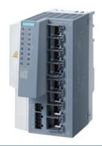
SCALANCE XCM108PoE (8x100/1000 Mbit/s RJ45, PoE) unmanaged IE Switch up to 120 W PoE power on 8 ports, LED diagnostics, error-signaling contact with set pushbutton, redundant power supply manual available as a download.
