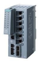
SCALANCE XC206-2SFP EEC manageable Layer 2 IE switch IEC 62443-4-2 certified; 6x 10/100 Mbit/s RJ45 ports; 2x 100/1000 Mbit/s SFP; 1x console port; diagnostics LED; redundant power supply; with painted printed-circuit boards; NAMUR NE21-compliant; temperature range -40 °C to +70 °C; assembly: DIN rail/S7 mounting rail/wall; redundancy functions; office features (RSTP, VLAN,...); PROFINET IO device; Ethernet/IP-compliant; C-PLUG slot;
