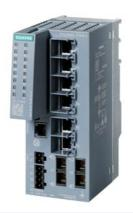
SCALANCE XC206-2 manageable Layer 2 IE switch; IEC 62443-4-2 certified; 6x 10/100 Mbit/s RJ45 ports; 2x 100 Mbit/s SC-ports, 1x console port; diagnostics LED; redundant power supply; temperature range -40 °C to +70 °C; assembly: DIN rail/S7 mounting rail/wall; redundancy functions; office features (RSTP, VLAN,...); PROFINET IO device Ethernet/IP-compliant C-PLUG slot.
