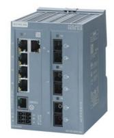
SCALANCE XB205-3LD managed layer 2 IE switch 5x 10/100 Mbit/s RJ45 ports 3x SM FO SC-port 1x console port, diagnostics LED redundant power supply; IEC 62443-4-2 certified; temperature range 0 °C to +60 °C; DIN-rail mounting; default EtherNet/IP.
