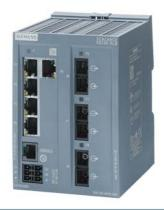
SCALANCE XB205-3LD managed layer 2 IE switch 5x 10/100 Mbit/s RJ45 ports 3x SM FO SC-port 1x console port, diagnostics LED redundant power supply; IEC 62443-4-2 certified; temperature range 0 °C to +60 °C; DIN-rail mounting; default PROFINET.
