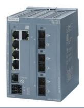
SCALANCE XB205-3 managed Layer 2 IE Switch 5x IEC 62443-4-2 certified; 10/100 Mbit/s RJ45 ports 3x MM FO SC-port 1x console port, diagnostics LED redundant power supply; IEC 62443-4-2 certified; temperature range 0  $^{\circ}\text{C}$  to +60  $^{\circ}\text{C}$ ; DIN-rail mounting; default EtherNet/IP.
