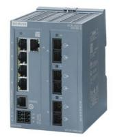
SCALANCE XB205-3 managed Layer 2 IE switch 5x 10/100 Mbit/s RJ45 ports 3x MM FO SC-port 1x console port, diagnostics LED redundant power supply; IEC 62443-4-2 certified; temperature range 0 °C to +60 °C; DIN-rail mounting; default PROFINET.
