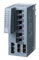
SCALANCE XC106-2, Unmanaged IE switch, 6x 10/100 Mbit/s RJ45 ports, 2x 100 Mbit/s Multimode SC, LED diagnostics, error-signaling contact with set pushbutton, redundant power supply Manual available as a download .
