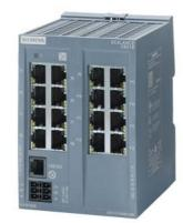
SCALANCE XB216 managed Layer 2 IE switch, 16X 10/100 Mbit/s RJ45 ports, 1x console port, diagnostics LED red redundant power supply; IEC 62443-4-2 certified; temperature range 0 to +60 °C DIN-rail mounting; default EtherNet/IP.
