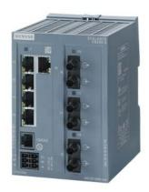
SCALANCE XB205-3 managed Layer 2 IE switch 5x 10/100 Mbit/s RJ45 ports 3x MM FO ST port 1x console port, diagnostics LED redundant power supply; IEC 62443-4-2 certified; temperature range 0 °C to +60 °C; DIN-rail mounting; default PROFINET.
