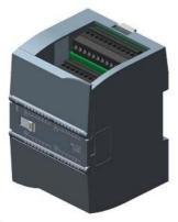
SIPLUS S7-1200 SM 1223 16DI/16DQ RLY based on 6ES7223-1PL32-0XB0 with conformal coating, -40...+70  $^{\circ}$ C, start up -25  $^{\circ}$ C, digital input/output 16 DI/16 DQ, 16 DI 24 V DC, sink/source, 16 DQ, relay 2 A
