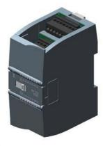
SIPLUS S7-1200 SM 1223 8DI/8DQ based on 6ES7223-1BH32-0XB0 with conformal coating, -40...+70 °C, start up -25 °C, digital input/output SM 1223, 8 DI/8 DQ, 8 DI 24 V DC, sink/source, 8 DQ, transistor 0.5 A
