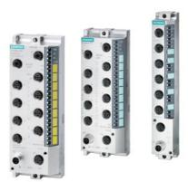
SIMATIC DP, ET 200eco PN, F-DI 8x24 V /F-DQ 3x24 V 2 A, M12 PROFIsafe, up to PL e (ISO 13849), up to SIL 3 (IEC 61508), degree of protection IP65/67, including eCoding plug-in connector
