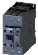
power contactor, AC-3e/AC-3, 65 A, 30 kW / 400 V, 3-pole, 20-33 V AC/DC, 50/60 Hz, with integrated varistor, auxiliary contacts: 1 NO + 1 NC, screw terminal, size: S2
