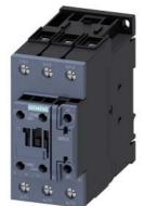
power contactor, AC-3e/AC-3, 51 A, 22 kW / 400 V, 3-pole, 24 V AC, 50 Hz, auxiliary contacts: 1 NO + 1 NC, screw terminal, size: S2  $\,$
