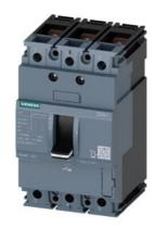
circuit breaker 3VA1 IEC frame 100 breaking capacity class B Icu=16kA @ 415V 3-pole, line protection TM210, FTFM, In=50A overload protection Ir=50A fixed short-circuit protection Ii=10 x In nut keeper kit
