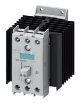
Solid-state contactor 3-phase 3RF2 AC 51 / 20 A / 40  $^{\circ}$ C 48-600 V / 4-30 V DC 3-phase controlled screw terminal Blocking voltage 1200 V
