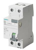
Residual current operated circuit breaker, 2-pole, Type AC, In: 25 A, 30 mA, Un AC: 230 V  $\,$
