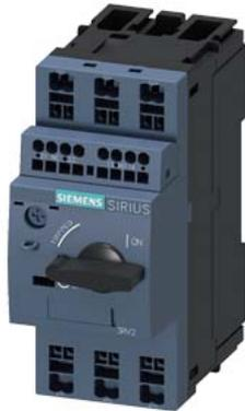
Circuit breaker size S00 for motor protection, CLASS 10 A-release 0.55...0.8 A N-release 10 A Spring-type terminal Standard switching capacity with transverse auxiliary switches 1 NO+1 NC
