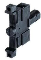
COMPONENT FOR ENCLOSURE, 22MM LAMP HOLDER WITH INTEGRATED LED 24V AC/DC RATED VOLTAGE 24V AC/DC SCREW TERMINAL YELLOW !!! Phased-out product !!! SIRIUS ACT 3SU1 is successor Preferred successor type is >>3SU1401-2BB30-1AA0<<
