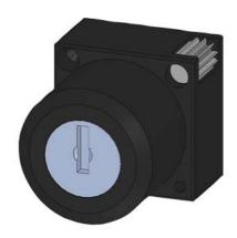
RONIS KEY-OPERATED SWITCH, 22MM, ROUND, PLASTIC, LOCK NO. SB30, WITH 2 KEYS, 2 SWITCH POSITIONS O-I, LATCHING, ACTUATING ANGLE 50 DEG.,12/14H, KEY REMOVAL POS. I, WITH HOLDER, POSSIBLE SPECIAL LOCKS: SB31, 421, 455 !!! Phased-out product !!! SIRIUS ACT 3SU1 is suc Preferred successor ty >>3SU1000-4BF21-0AA0 + 3SU1500-0AA10-0AA0<<
