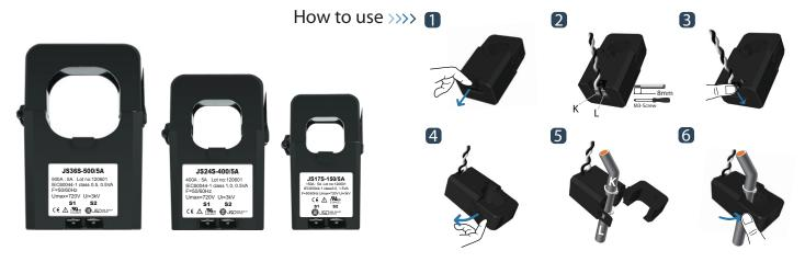
JS series of split-core current transformer offers 5A at secondary from sensed primary current for metering application. It can be used for power meter, distribution system, control panels, switchgear and other equipment. It is designed to install to live power line without disconnection as split-core compact type. Also, over-voltage protection circuit is included to offer safe, fast and cost effective installation.
