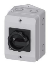
SENTRON, Switch disconnector 3LD, main switch, 3-pole, lu: 25 A, Operating power / at AC-23 A at 400 V: 9.5 kW, molded-plastic encapsulation for metric screw connection, 1 NC, 1 NO, rotary operating mechanism, black
