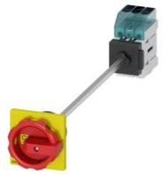
Load disconnector 3LD3, lu 63 A Main switch 3-pole Rated operating capacity at AC-23 A at 400V 22.0 kW floor mounting Basic switch with door coupling Central hole mounting 22.5mm Rotary actuator red / yellow 66 x 66 mm
