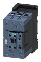
power contactor, AC-3e/AC-3, 95 A, 45 kW / 400 V, 3-pole, 20-33 V AC/DC, 50/60 Hz, with integrated varistor, auxiliary contacts: 1 NO + 1 NC, screw terminal, size: S3  $\,$
