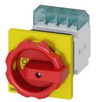
SENTRON, Switch disconnector 3LD, emergency switching-off switch, 3- pole, lu: 16 A, operating power / at AC-23 A 400 V: 7.5 kW, front-mounted, rotary operating mechanism, Red / yellow, central mounting 22.5 mm of the handle
